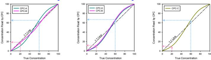
If CPCs have poor linearity, PCRF determined by the CPCs will have errors. If two CPCs have the linearity curves above, comparison between the two tells that something is wrong in the linearity, at least in one of the two CPCs.
