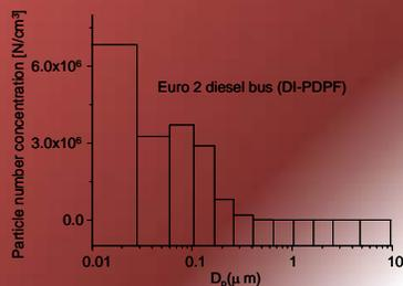
Figure 1. Measured diesel particulate number concentrations from Euro 2 diesel city bus with pDPF catalyst during Braunschweig City Driving Cycle.
