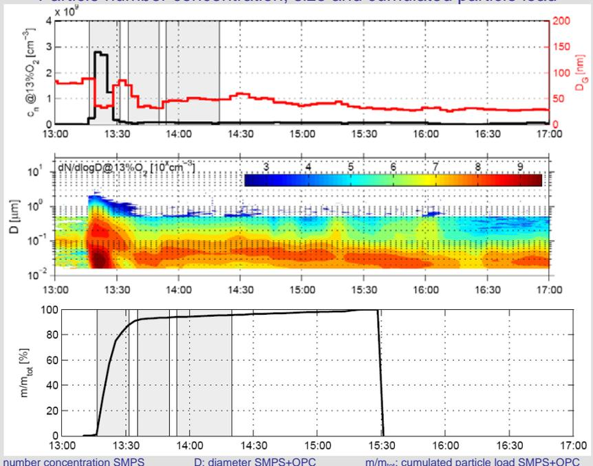
$c_n$ : number concentration SMPS      D: diameter SMPS+OPC       $m/m_{tot}$ : cumulated particle load SMPS+OPC
