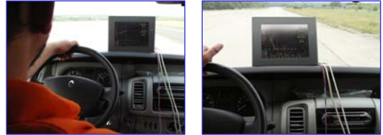
When replicating a drive cycle, the driver is operating a vehicle to match the actual speed to the cycle speed, just like on a chassis dynamometer.
