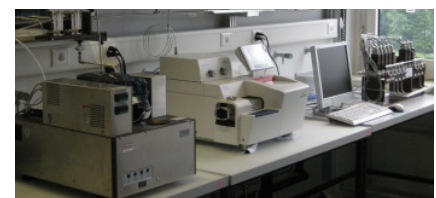
Overview of the TGA-FTIR system
