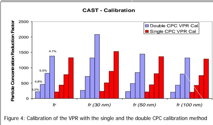
Figure 4: Calibration of the VPR with the single and the double CPC calibration method
