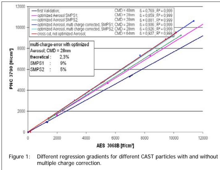
Figure 1: Different regression gradients for different CAST particles with and without multiple charge correction.
