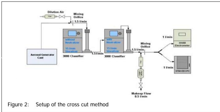
Figure 2: Setup of the cross cut method
