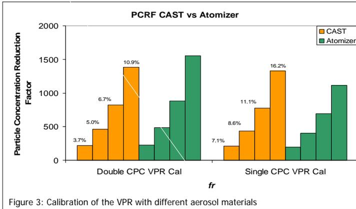
Figure 3: Calibration of the VPR with different aerosol materials
