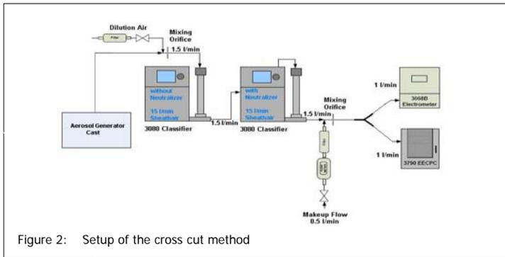
Figure 2: Setup of the cross cut method
