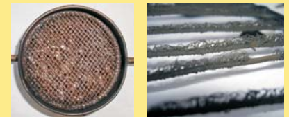
Dedusting and conversion lattice Soot collection
