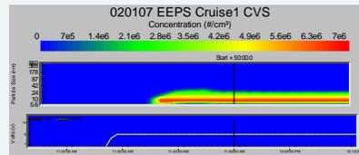
Figure 4. Results Particle Size Distribution - Cruise. Vanadium-based SCR catalyst. Here we see the delay between reaching top speed (50mph) and the onset of the nucleation mode, which does not set in until the exhaust temperature out of the SCR catalyst has reached approximately 310°C.
