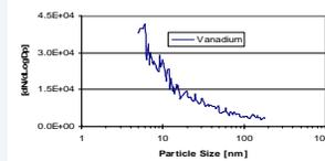
Figure 8. Average Particle Size Distribution. Idling operation. Particle concentrations are comparable to tunnel blanks. Similar for both vanadium and zeolite systems.
