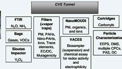
Figure 3. Emission Characterization Scheme. Sample collection of dilute exhaust from the CVS tunnel for physical, chemical, and toxicological characterization.
