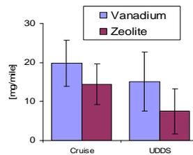
Figure 2. Preliminary PM Mass and NO<sub>x</sub> Emissions. The Vanadium-based system more effectively converts SO<sub>2</sub> to SO<sub>3</sub>, and therefore emits more sulfate and PM overall. The activation temperature window for the two NO<sub>x</sub> catalysts is shown in the insert.
