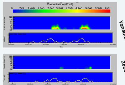
Figure 5. Results Particle Size Distribution - UDDS. Here are the EEPS results for the vanadium and zeolite systems over the UDDS cycle. The speed trace can be seen below. The two figures (Fig 4 and 5) are shown on the same scale to highlight the much larger nucleation mode with the vanadium system.
