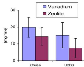
Figure 2. Preliminary PM Mass and NO<sub>x</sub> Emissions. The Vanadium-based system more effectively converts SO<sub>2</sub> to SO<sub>3</sub>, and therefore emits more sulfate and PM overall. The activation temperature window for the two NO<sub>x</sub> catalysts is shown in the insert.
