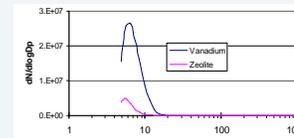
Figure 7. Average Particle Size Distribution. UDDS cycle. The nanoparticle emissions from the vanadium-based system are higher than the zeolite-based system due to the lower nucleation activation temperatures required.
