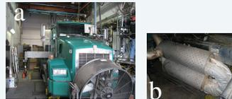
Figure 1. (a) Vehicle testing conducted at the CARB HDVEL. This test vehicle is a 1998 Class 8 Truck (>300K miles) powered by a Cummins M11 and equipped with a PM-NO<sub>x</sub> retrofit. (b) PM-NO<sub>x</sub> Retrofit. Tested in two versions for NO<sub>x</sub> control: (1) Vanadium-based catalyst and (2) Zeolite-based catalyst.
