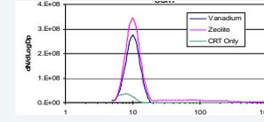
Figure 6. Average Particle Size Distribution. 50 mph Cruise. Size distributions are similar for both SCR systems. Notice the much diminished nucleation mode for a CRT system.
