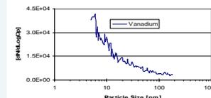
Figure 8. Average Particle Size Distribution. Idling operation. Particle concentrations are comparable to tunnel blanks. Similar for both vanadium and zeolite systems.
