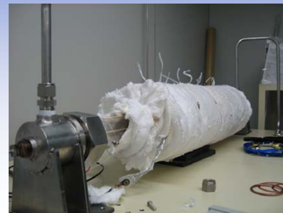
Fig. 2 A picture of flow reactor used in this study.
