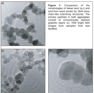
The average diameter of primary particles (D) from diesel exhaust vehicles is smaller than the average D from wood smoke (Table 1). The average D from ambient samples from Zurich and from Roveredo in summer are approximately the same as those from diesel exhaust, the average D from ambient samples from Roveredo in winter are slightly smaller than those from wood smoke.
