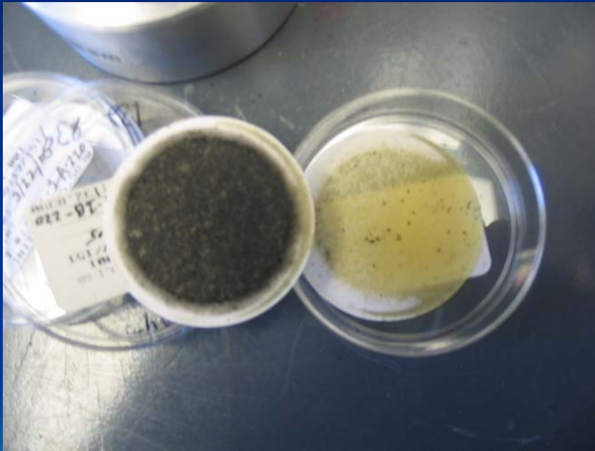
Primary and Backup Filter
