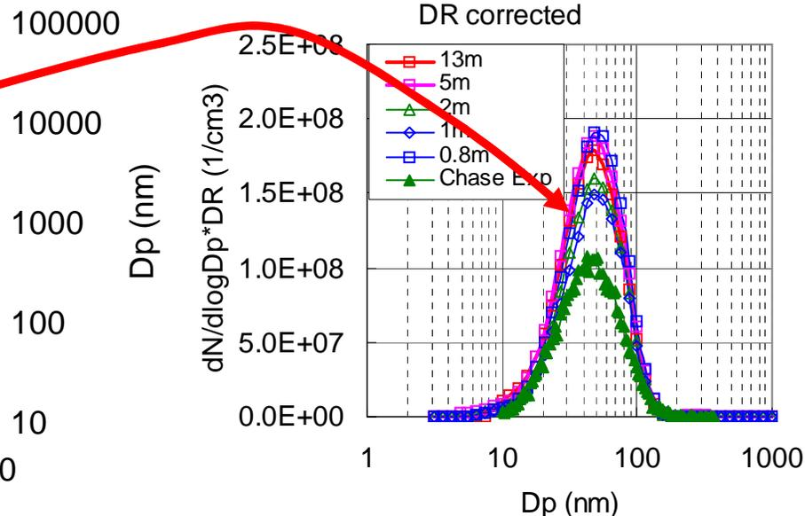
Particle size distribution corrected with dilution ratio are **metastable** at **DR (dilution ratio)  $\geq 5$** .
