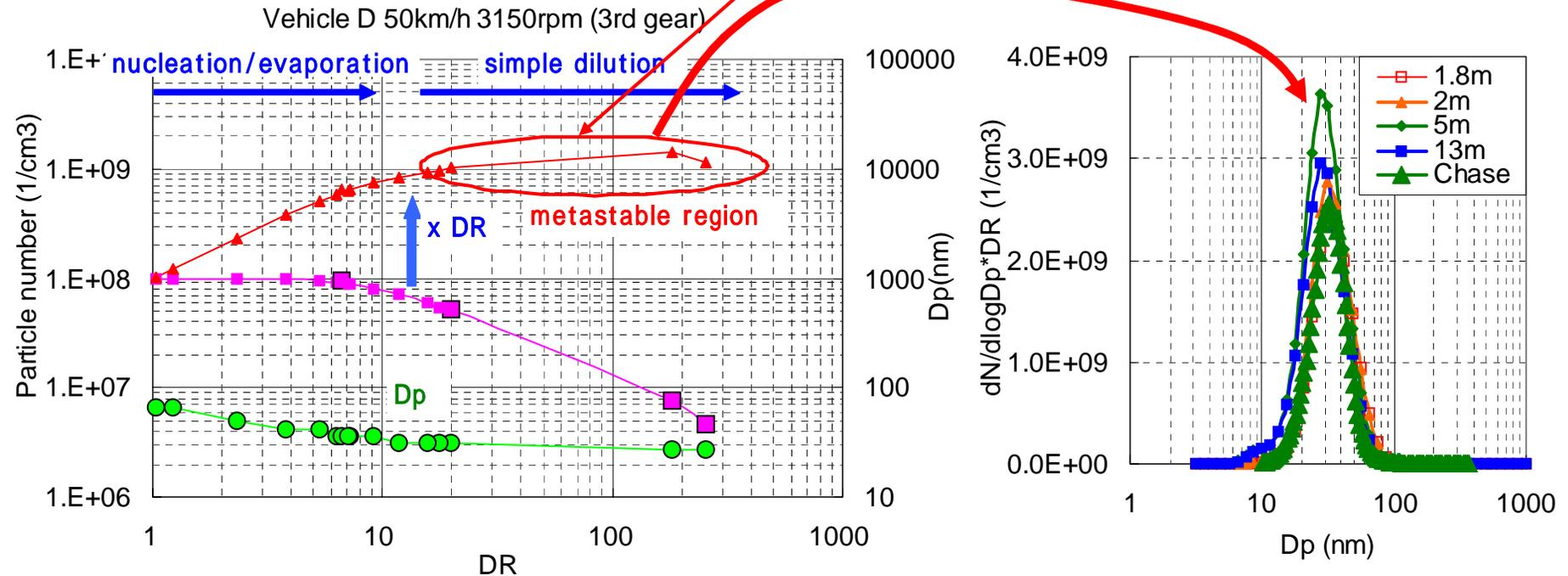
**Particle size distribution was approximately unchanged at >2m behind the tail pipe (DR >18).**
