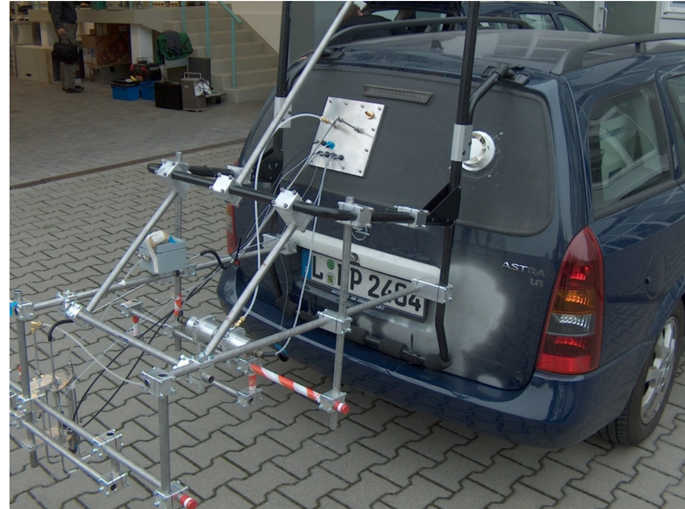
Inlet system used in this project: SMPS, exhaust gas, humidity, temperature and flow velocity measurements are taken at adjustable locations within the exhaust plume on public roads
