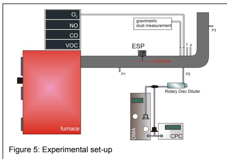
Figure 5: Experimental set-up
