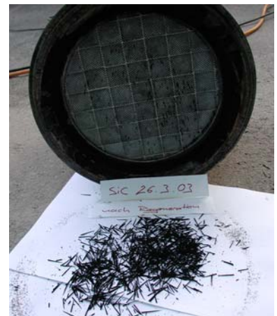
Fig. 1: soot-bars after regeneration ("French fries")
