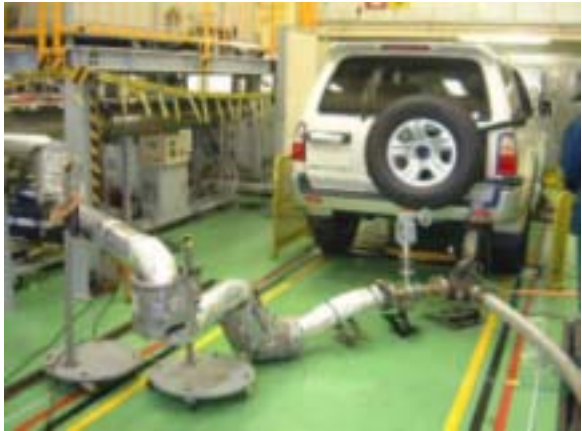
Test vehicle and Dilution tunnel
