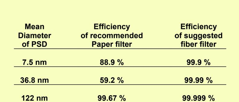
Filter efficiency for different particle diameters
