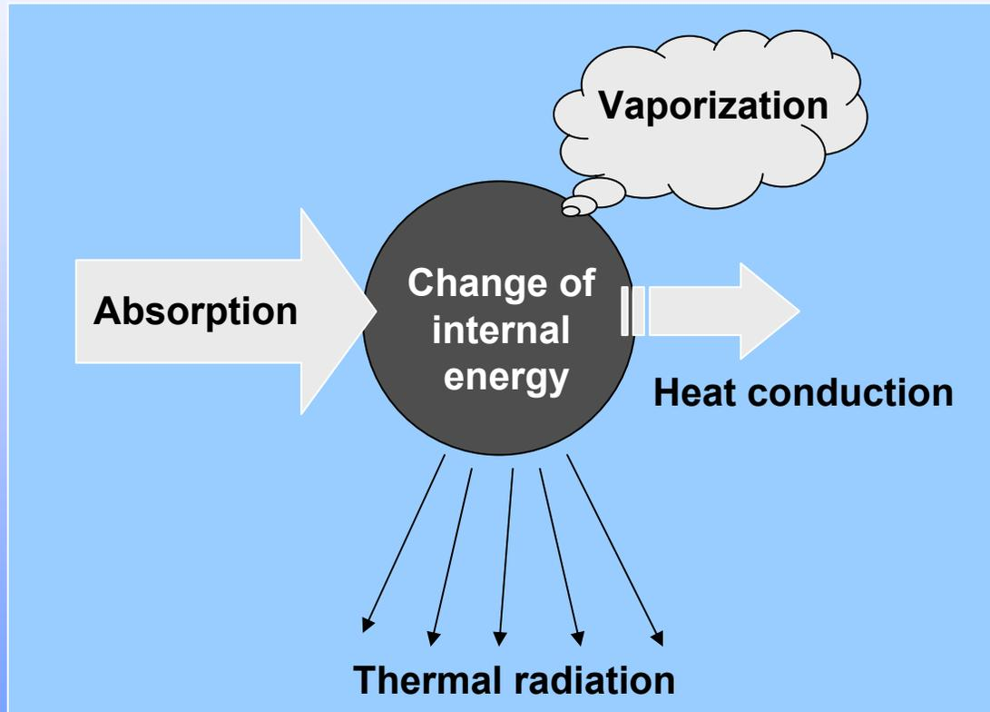
$$\underbrace{Q_{abs} \cdot \frac{\pi d_p^2}{4} \cdot E_i}_{Absorption} - \underbrace{\Lambda \cdot (T - T_0) \cdot \pi d_p^2}_{Heat\ conduction} + \underbrace{\frac{\Delta H_v}{M} \cdot \frac{dm}{dt}}_{Vaporization} - \underbrace{\pi d_p^2 \int \varepsilon(d_p, \lambda) M_\lambda^b(T, \lambda) \cdot d\lambda}_{Thermal\ radiation} - \underbrace{\frac{\pi d_p^3}{6} \rho_s \cdot C_s \cdot \frac{dT}{dt}}_{Change\ of\ internal\ energy} = 0$$
