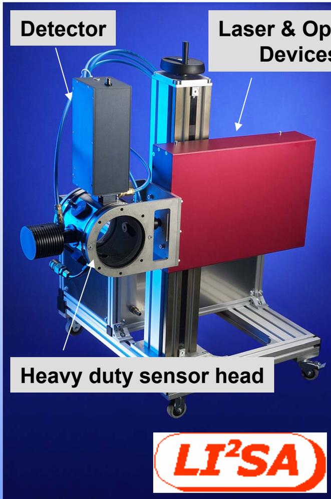
Direct integration of an adapter ring into the raw exhaust pipe on chassis dynamometers and motor test benches possible (full flow sensor head)
