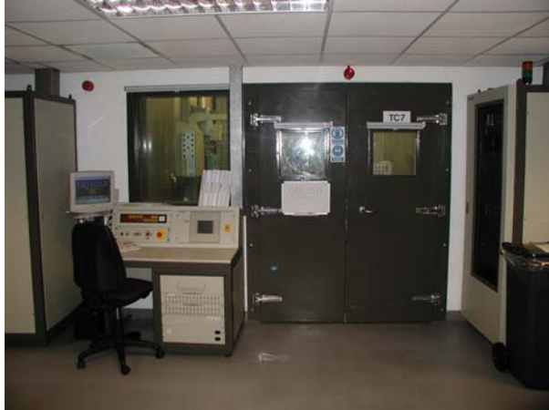
Figure 2 The outside of the test cell housing the VW TDi. The control panel can be seen on the left.
