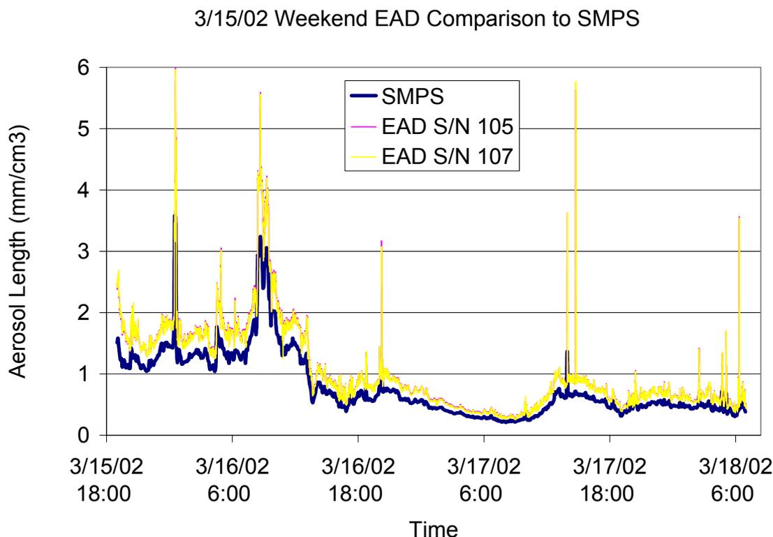
**Figure 12 Atmospheric Aerosol comparing SMPS and EAD length data**
