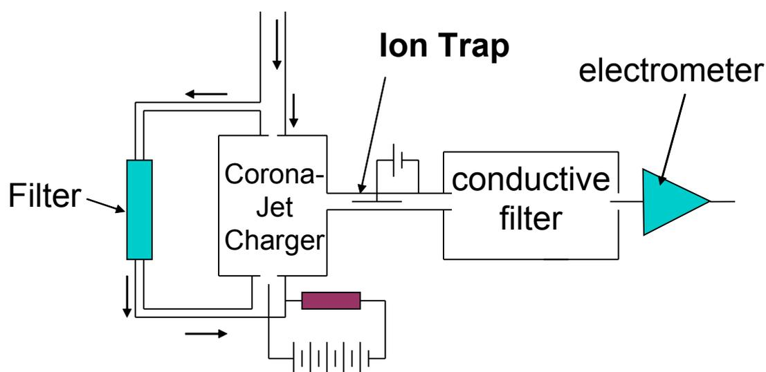
Figure 3 EAD Charger and Ion Trap
