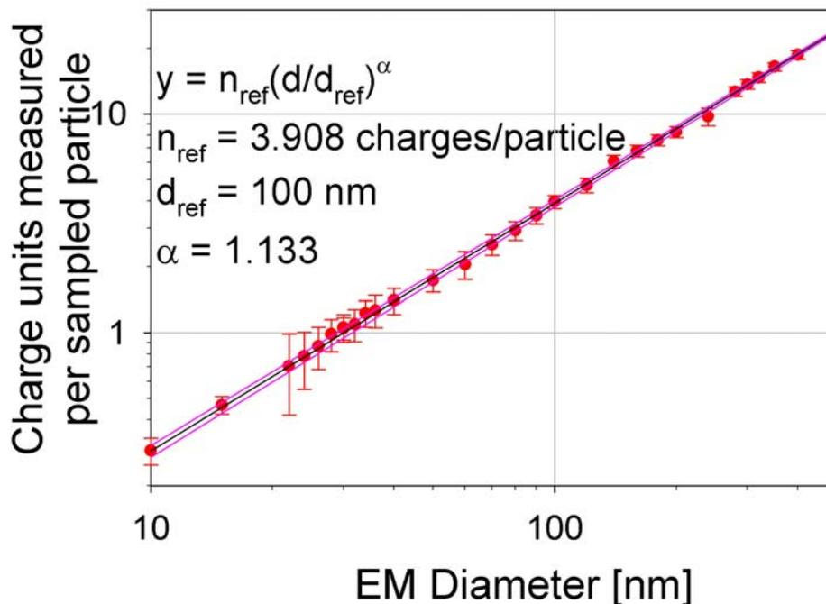
Figure 6 Electrical Aerosol Detector overall response
