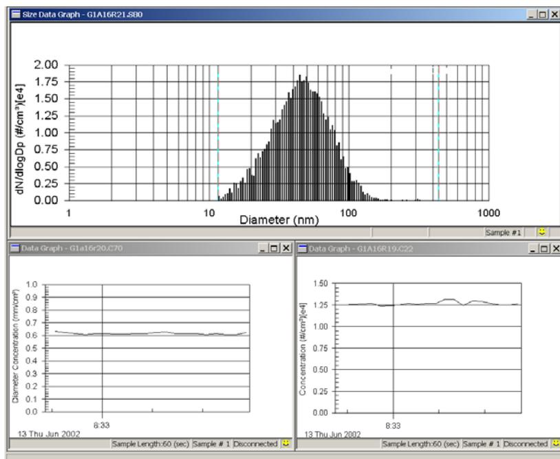
**Figure 9 Measurements from CAST aerosol source on SMPS, EAD and CPC**
