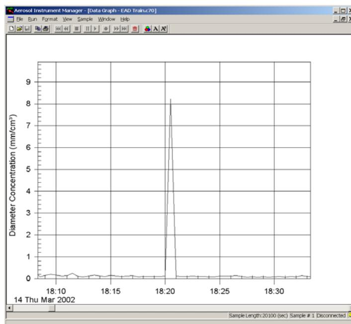
Figure 11 Diesel train passes TSI monitoring station - EAD data
