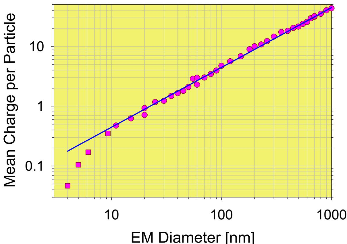
Figure 5 Measured Charge per Particle versus Electrical Mobility Diameter for Charger
