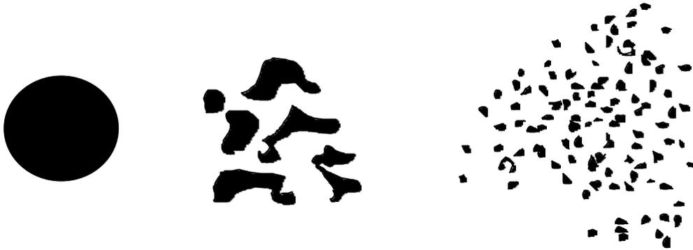
Graphical representation of turbulent and diffusive mixing of an exhaust clump
