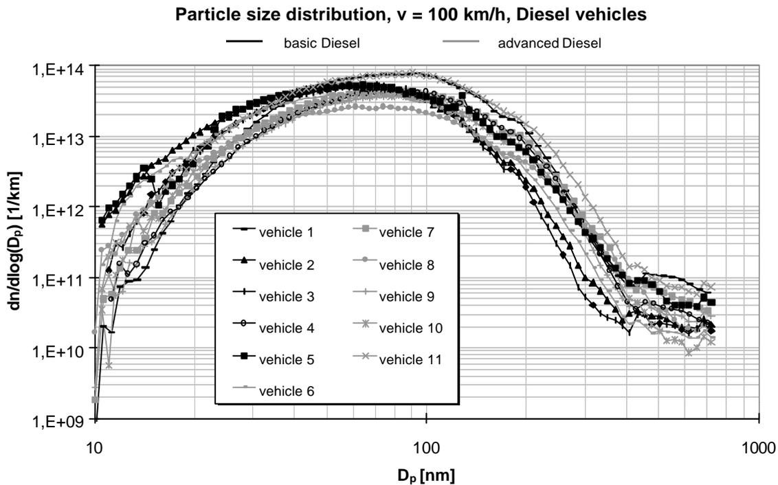
Fig. 1: Particle size distribution of Diesel engines measured at a constant speed at 100 km/h
