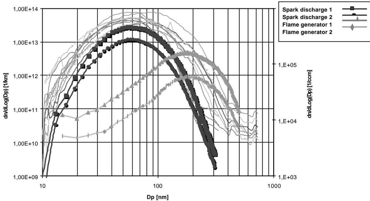
Fig. 3: Comparison of the test aerosol size distributions with emission data
