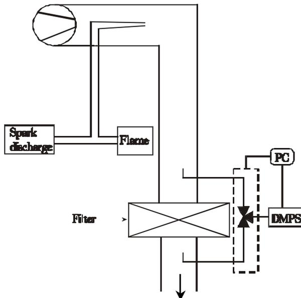
Fig. 4: The filter test block
