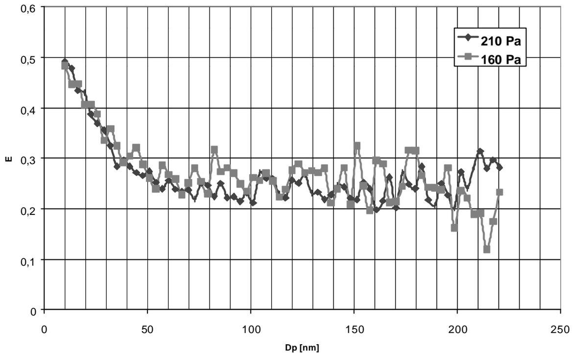
Fig. 4: Filter Efficiency E vs. particle mobility diameter ( $4,7 \text{ m}^3/\text{min}$ )
