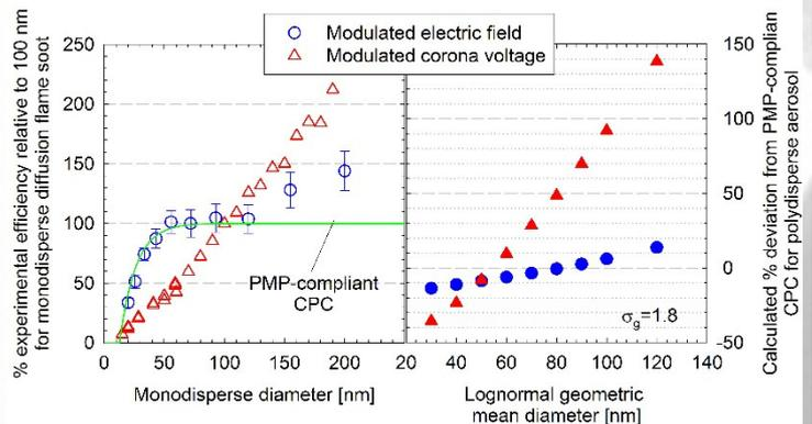
Figure 2: Left-hand panel: Experimentally determined size dependence on monodisperse soot particles for the original particle detector (modulated corona voltage) and a prototype one (modulated electric field) developed for the PN-PEMS. Right-hand panel: Calculated correlation of the two sensors against the a PMP-compliant CPC for polydisperse lognormal distributions (geometric standard deviation of 1.8).
